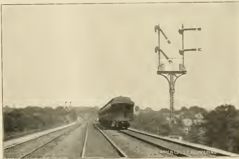
SIGNALS GOVERNING RIGHT-HAND TRACK, PROTECTING REAR OF TRAIN WHICH HAS JUST PASSED.
